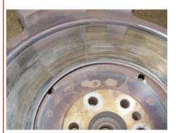
Even though a used flywheel may have the appearance of being perfectly flat, always have it machined to remove the hard surface, and restore it to the same finish and friction value, as the new clutch pressure plates to be installed.
