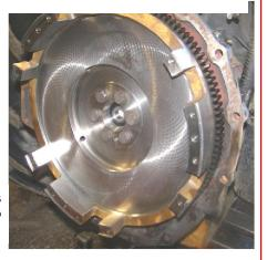
When refacing a flywheel it is essential that any location steps and pot depths are re-established to the correct dimensions to ensure correct operation of the clutch.
